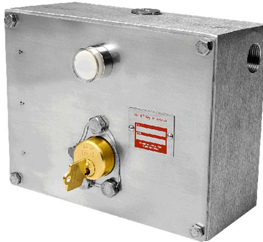
The Type SKRU consists of an interlock, a solenoid, and an auxiliary switch. The solenoid is designed to permit removal of the interlock key in response to an external electric signal. The auxiliary switch is a quick-make, quick-break device, which operates when the interlock key is rotated. Normally, the key is trapped in the SKRU and the solenoid is de-energized. To release the key, a signal must be sent to the solenoid from an external source.
